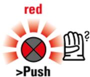
**Measuring errors** caused, for example, by the wearing a glove when switching on are indicated by the signal unit **flashing RED**. In this case, the PRCD-S<sup>+</sup> from PCE gives a visual warning and does not switch on. After acknowledging the fault, repeat the starting procedure without a glove or after changing your location.
