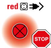
If, when switching on, the signal unit **illuminates RED or remains neutral** within approx. 2 sec., there is a **fault**. The PRCD-S<sup>+</sup> does not switch ON. Consult a qualified electrician
